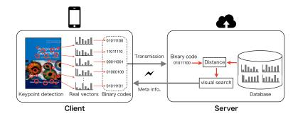
Fig. 1. Our system framework in client server system.
